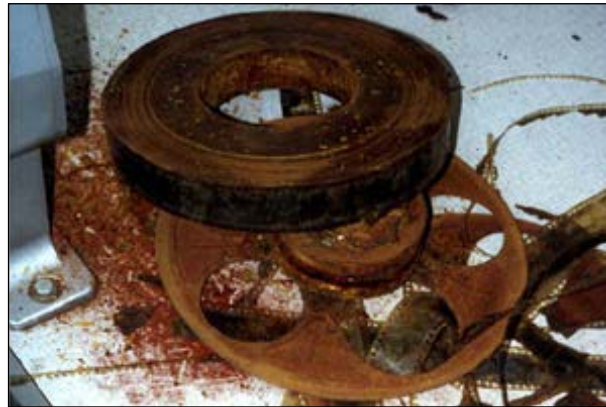
Figs. 3-5: Nitrate film in various states of decay.
